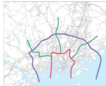
Fig. 5. A more extensive impact assessment was conducted using the gate zone model (VEI). The model includes three radial cordons in addition to the cordons within ring roads I and III. The impact assessment was made in the 2025 situation with investments outlined in HSL 2015.
